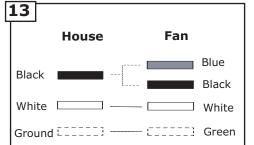
Connect black and blue wire from fan to Black or (Hot) wire from house. Connect White wire from Fan to White (Neutral) wire from house. Connect Ground leads from mounting bracket and downrod to Ground lead from house. Refer to Safety Tips section of manual.
